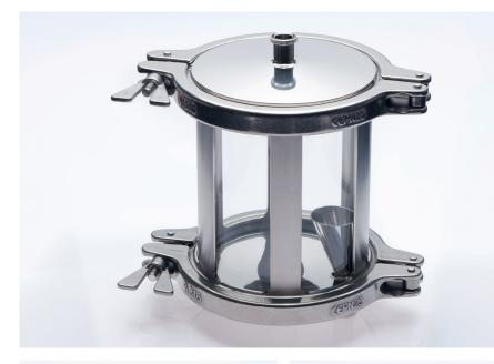
The **CT-Bubble Trap** (Patent Pending) has been developed to incorporate the best features of the ACL Bubble Trap and the CT-SVFI (patent pending). The glass/o-ring/flange end is sealed utilising a sanitary clamp. As there is a mechanical stop, the gasket cannot be overcompressed. The use of a clamp connection reduces the need for tools to assemble or disassemble the bubble trap. Additional seals provide a secondary barrier to prevent the ingress of contaminants to the seal location.
